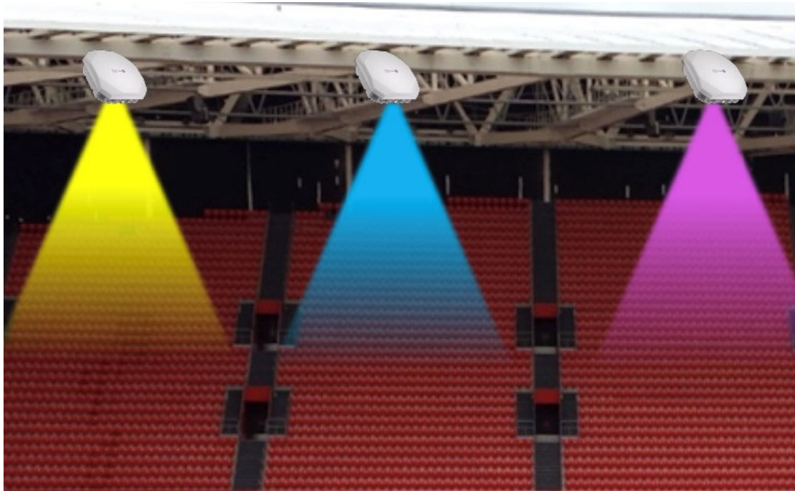
Figure 19: AP installation on the steel frames on the stadium roof
